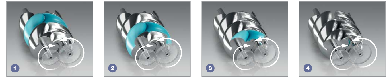
1 Intake air is captured 2 Volume is reduced 3 Expelled to pressure side 4 Flow chamber completely evacuated
